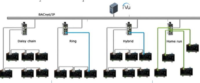
Require Ethernet switches with spanning tree protocol feature
